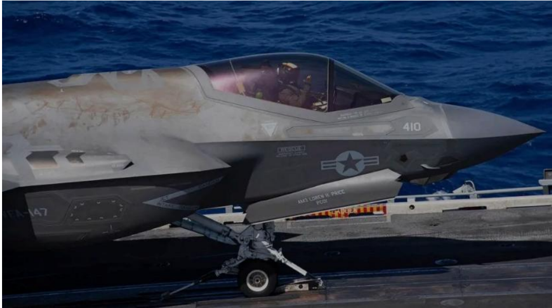
F35B on deck showing signs of corrosion causing discolouration – Source: US Finds Solution to Corrosion Problem on F-35 Jets , Aeronaut Media 13 Jul 25
