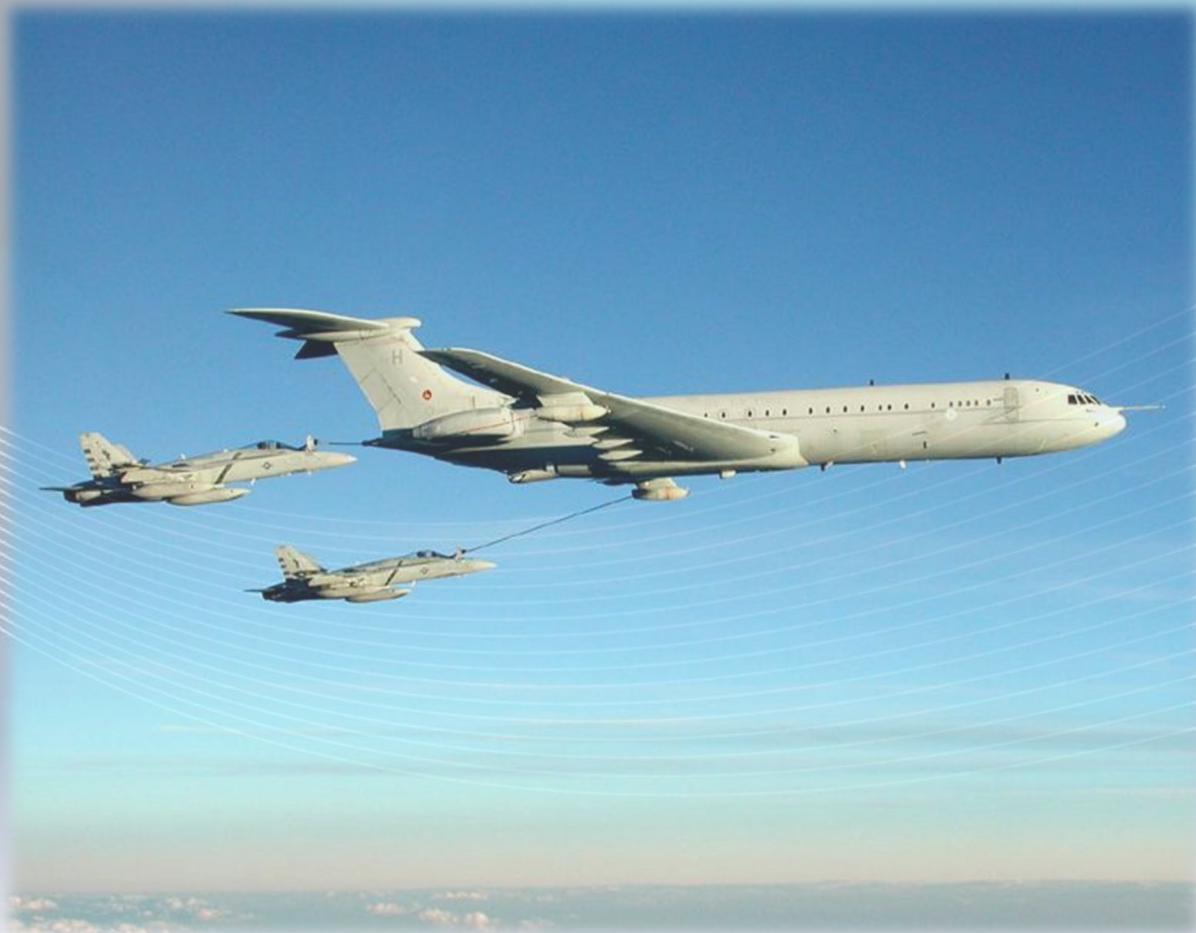
Pictured: U.S. F/A-18 Hornets received fuel from British VC-10 tanker due in part to STANAG 3447, "Aerial Refueling Equipment"
